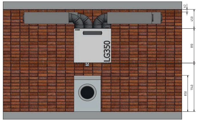
Wall-mounted installation with air exchange silencers
